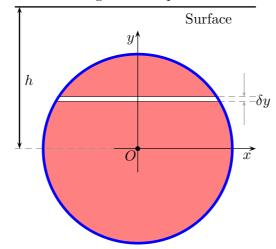
The second moment of inertia can be found by taking second moment of area about the plate's centreline along the x-axis and applying the parallel axis theorem.
